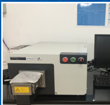
Equipment alloy analyzer (Emission spectroscopy technique) Model FM Smart
