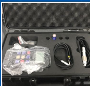
Equipment for checking thickness of paint
